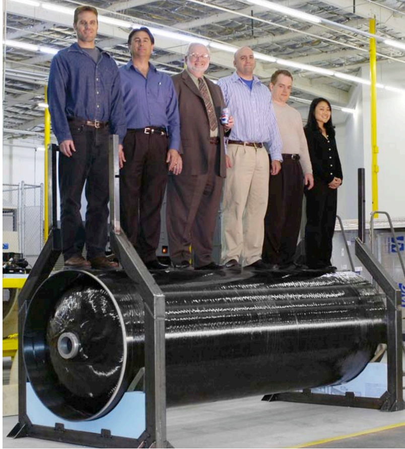
The Microcosm engineering crew is on top of their work. This is the prototype LOX tank for the Sprite Small Launch Vehicle, a member of the Scorpion ® family of responsive, low-cost launchers. From left, Dana, Keeler, Blake Bartosh, Jim Wertz, Aaron Leichner, John Collins, and Lynn Shimohara.
